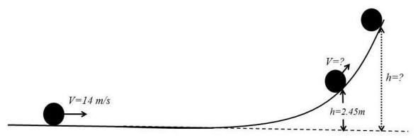
a) Calculate the speed of the ball when it is 2.45 m high?
